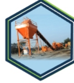
WET MIX DLC PLANT
