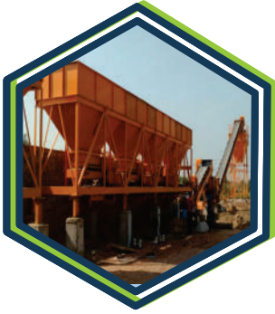
WET MIX MACADAM PLANT
