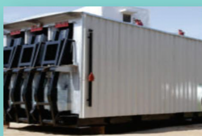
BITUMEN DRUM DECANDER
