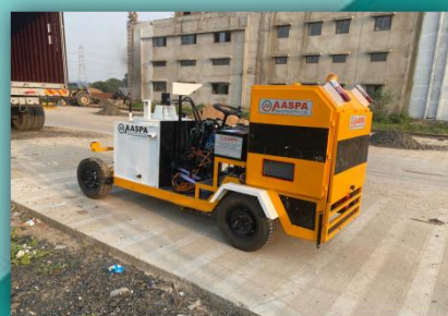
FULLY AUTOMATIC ROAD MARKING MACHINE
