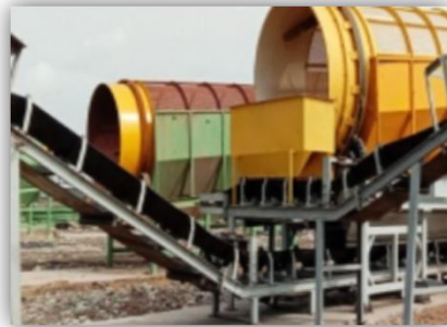
SEGRICATION COMPOST MACHINE
