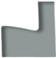
BARRIER KERB AND CHANNEL
