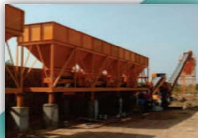
WET MIX MACADAM PLANT/DLC PLANT
