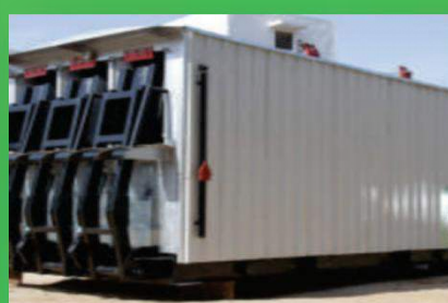
BITUMEN DRUM DECANDER
