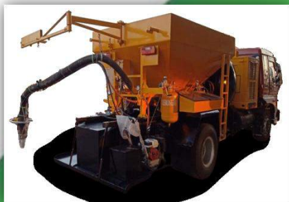
AASPA POTHOLE PATCHER WORKING PROCESS
