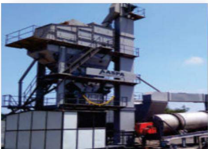
ASPHALT BATCH MIX PLANT
